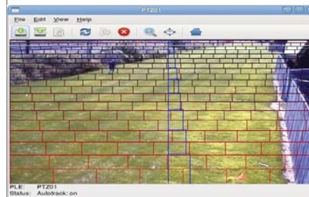
The AVT234 ® Horizon Line feature provides range and target estimates using proprietary calculations in place of need for range finders or GPS inputs.
